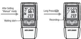
Fourth step: After recording some data, you can use the PC software download data. Sample rate is 1minute, 10 minutes is ten data.
