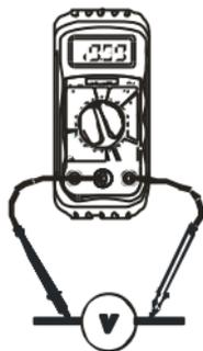
4. Read the voltage in the display. Reset the function switch to successively lower V DC positions to obtain a higher resolution reading. The display will indicate the proper decimal point and value. If the polarity is reversed, the display will show (-) minus before the value.
