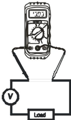
measurements, reset the function switch to successively lower mA DC positions to obtain a higher resolution reading. The display will indicate the proper decimal point and value.
